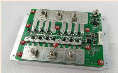
LN66 – 100A power board (150*100*33.5mm)
